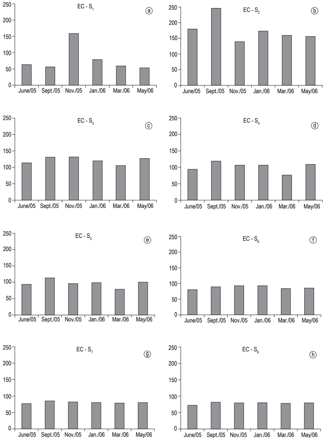
**Figure 3.** Electrical conductivity ( $\mu\text{S}\cdot\text{cm}^{-1}$ ) measures at each site and collection from the source to the mouth of Cintra Stream, Botucatu, São Paulo State, Brazil.
