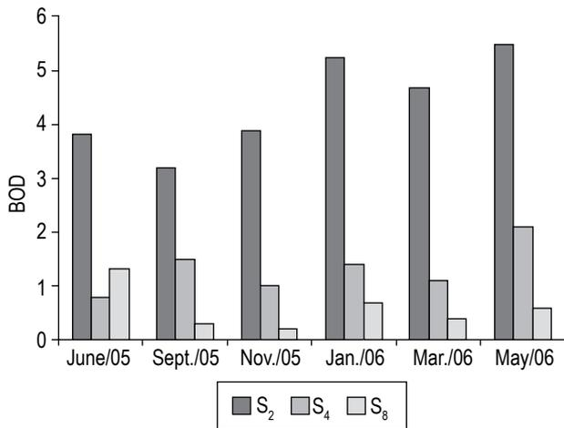
**Figure 7.** Biochemical oxygen demand ( $\text{mg.L}^{-1}$ ) at each site and collection from the source to the mouth of Cintra Stream, Botucatu, São Paulo State, Brazil.
