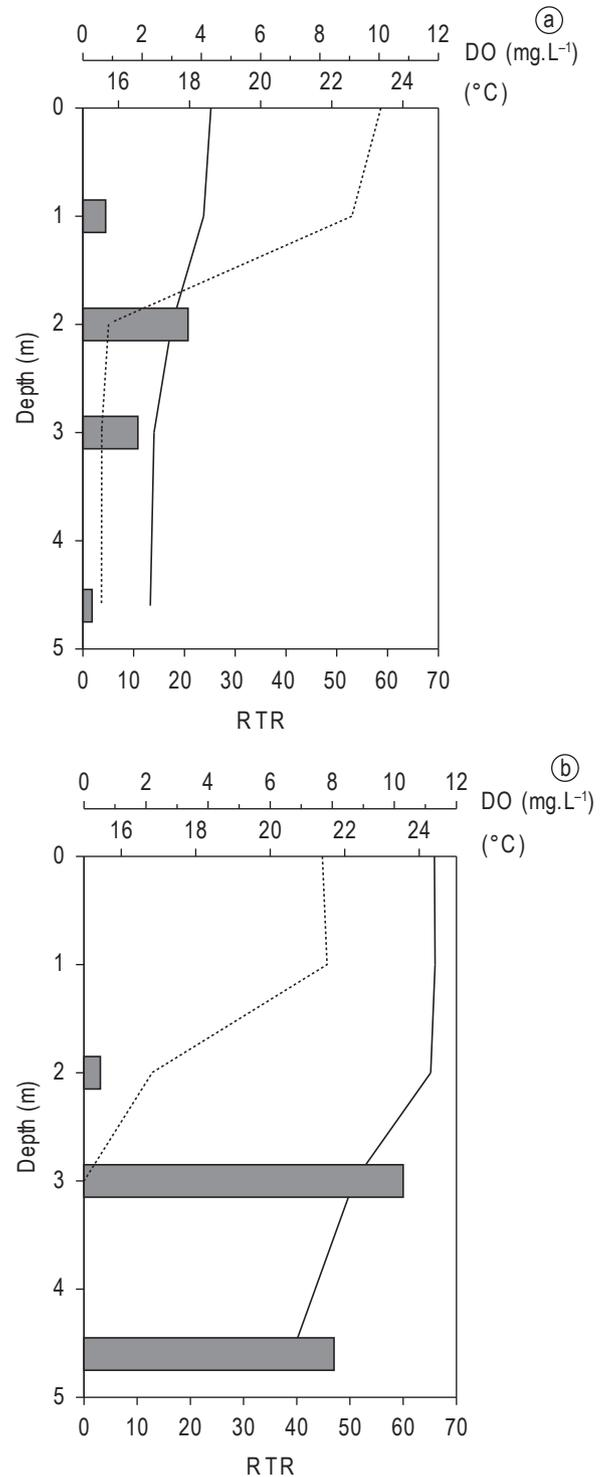
**Figure 2.** Vertical profile of mean values ( $n = 2$ ) for temperature (—), dissolved oxygen (---) and relative thermal resistance (RTR —) at Garças Reservoir during the a) dry a) and b) rainy period.
