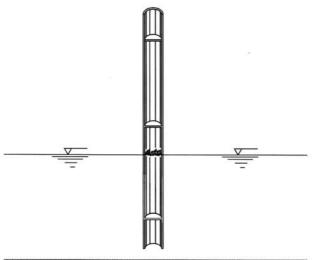
Figure 1: General view of the device used for collecting Chironomus xanthus in the field.
