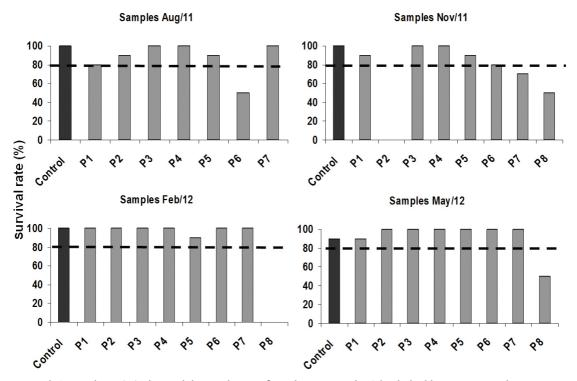
Figure 4. Survival rate (%) observed during the tests for sediment samples. The dashed line represents the minimum survival rate that must be achieved to express non acute effects.
