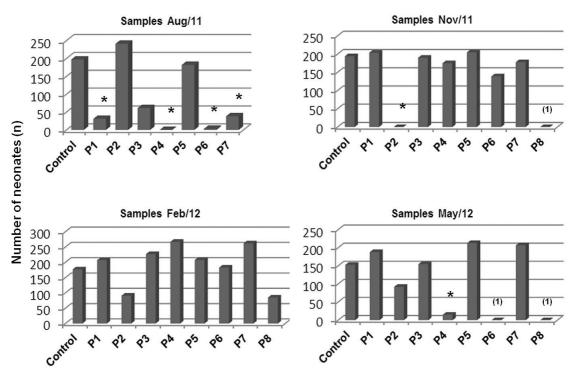
**Figure 3.** Total number of neonates (n) produced in each water sample during all sampling periods. The asterisk represents significant differences (p<0.05) compared to the negative control, showing chronic effect. (1) Without evaluation of chronic toxicity, because it showed 100% of acute mortality.
