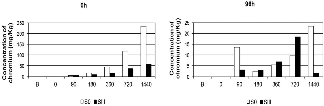
**Figure 3.** Chromium concentration in the sediment at the beginning (0h) and end (96h) of the tests with artificial sediment in *Chironomus xanthus* with (SIII) and without organic matter (S0). **B:** control (treatment with sand without contamination by chromium).
